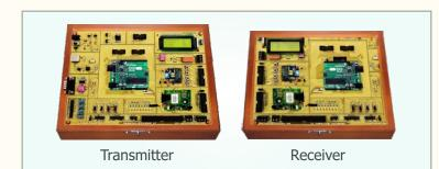
This trainer is used to send and receive sensor data by different wireless communication methods – like Bluetooth, Wifi, Zigbee, RF, GSM and GPS using Arduino Microcontroller.
