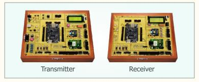
This trainer is used to send and receive sensor data by different wireless communication methods – like Bluetooth, Wifi, Zigbee, RF, GSM and GPS using Beaglebone Microcontroller.
